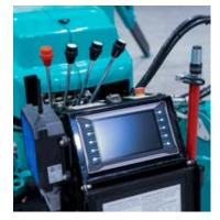
Manual control for arm folding/unfolding
